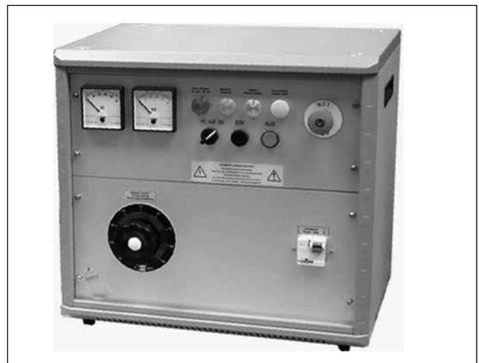
*Hi-Pot test is a contraction for high potential HV testing.*
